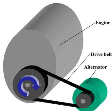
By connecting to an automotive cigarette lighter socket the measurement unit RPM-8000 senses the small AC ripple of the vehicle board net DC supply voltage and generates on its outputs both a TTL digital pulse train and an analog voltage signal. These signals are "per design" linear to the alternator RPM and by the linear drive belt relationship also to the engine RPM. The scaling factor can be determined by the relation between the effective diameters of the engine and the alternator pulleys.
