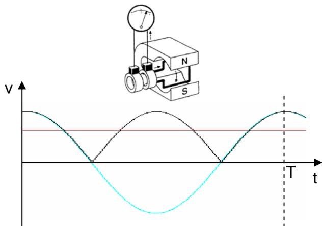
To imagine a three-phase generator we add two independent wire windings. Now we have 3 sine wave voltages which are spaced about  $120^\circ$  out of phase. After three-way rectification with six diodes the result is an alternating DC voltage with 6 pulses per revolution (black line) and an increased average voltage against the generator with one winding.
