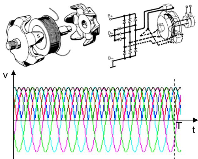
The board net voltage ripple frequency can simply be calculated by multiplying the alternator RPM with the number of poles (e.g. 12) and the number of phases (3).
