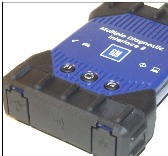
The GM MDI 2 is the next generation Global Diagnostic Interface tool for both current and future vehicles starting with Global A vehicles, and extending through future vehicle protocols and architectures. It's a compact communication module with increased processing power and security that manages the transfer of data between a vehicle's onboard ECU network with an auxiliary CAN bus.
